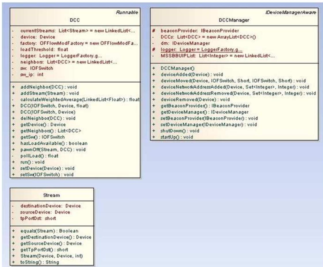
Figure 4.13: UML specification of DCC ClassObjects
