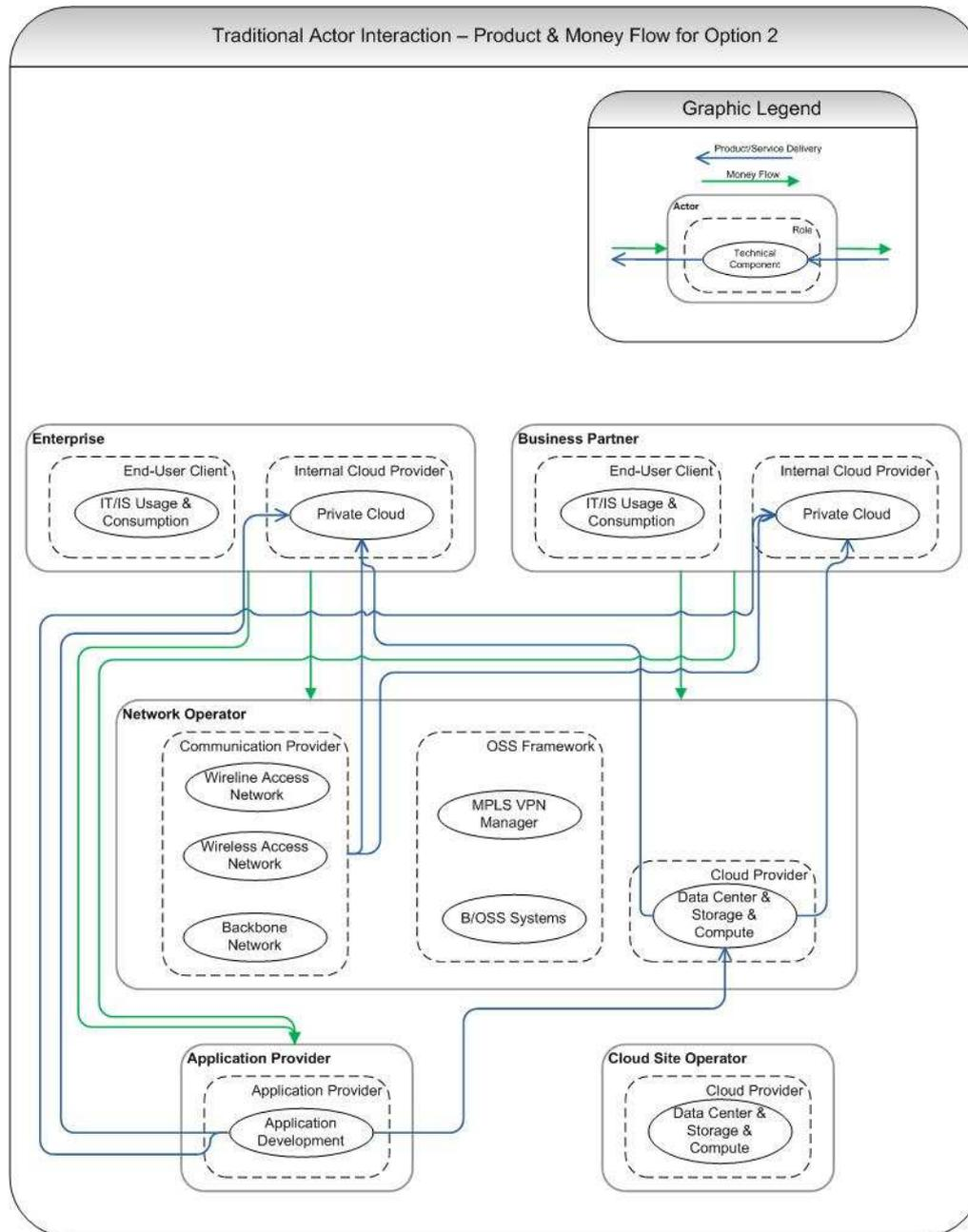
Figure 36. Network operator hosting VNC
