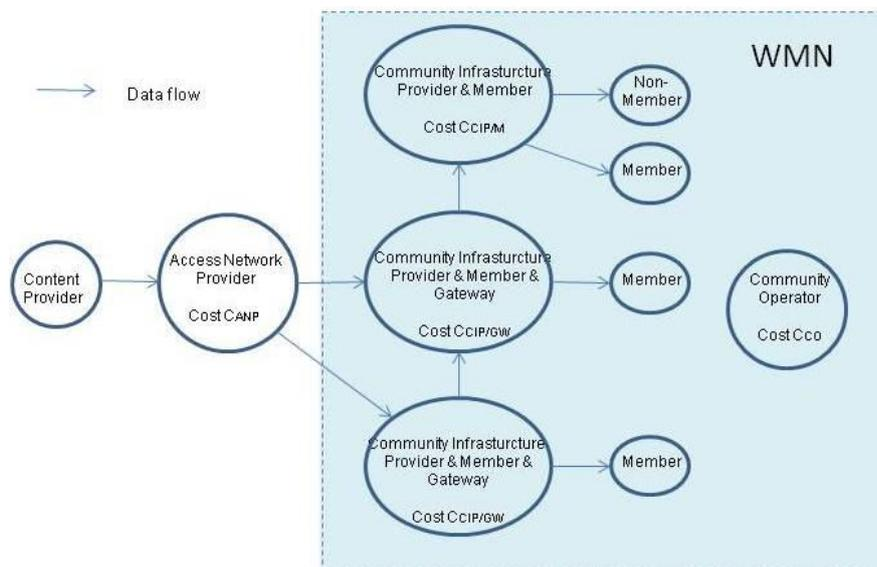
Figure 25. Data flows in Wireless Mesh Networks
