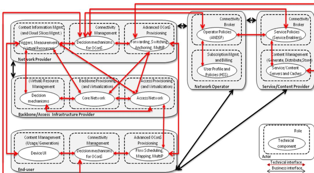
Figure 19. Network Architecture for OConS Use-Case 3 within OConS for CloNe [62].
