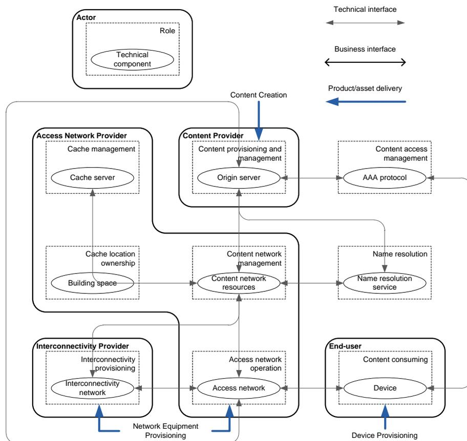
**Figure 9.** Value Network Configuration for ANP-centric NetInf architecture.
